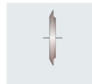
Pressing roll, 60 degrees, 3 cm layer
