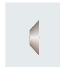
Pressing roll, 45 degrees, 12 cm layer
